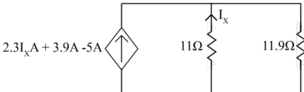
Note that the current controlled current source depends upon the current flowing through the 11Ω resistor, that is why it cannot be combined with the 11.9 Ω resistor, also because we need to find  $I_x$ .
