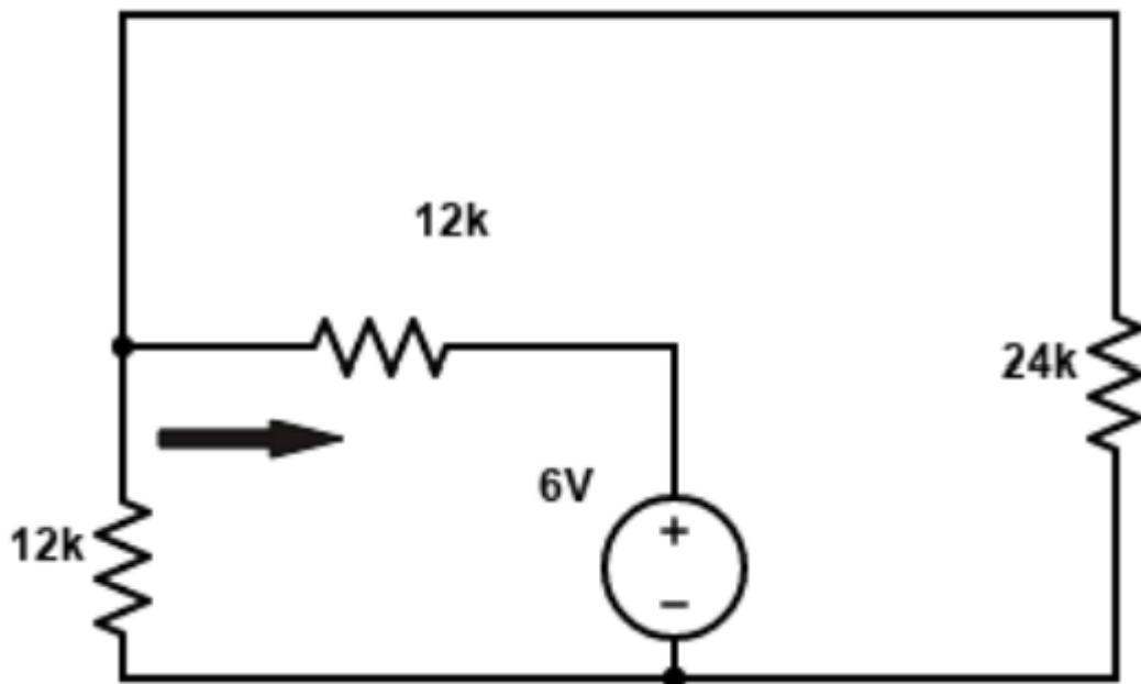
Simplify the resistors in parallel,
