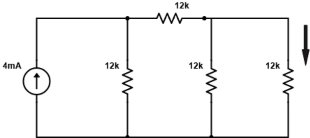
Consider the first two divisions(blue and pink) of the current in the figure below, the current for the blue arrow  $I_{blue}$  is (using current divider rule),
