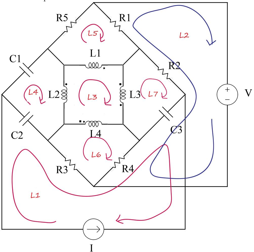
(ii) Use loop analysis. There are 8 nodes and 5 complete loops, so loop analysis will yield less equations making it.
