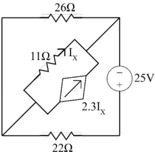
Apply Source Transformation on the series voltage source and resistor. i.e. (25V-22Ω).
