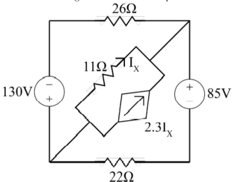
Apply Source Transformation again on all series voltage sources and resistors i.e. (130V-26Ω), (85V-22Ω).
