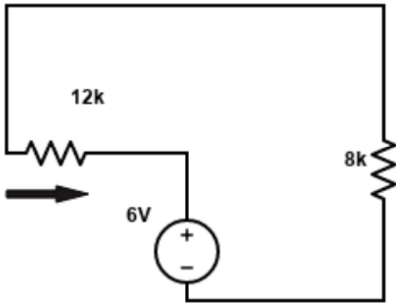
Notice the polarity of the voltage source and the direction of the current
