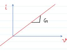
Slope of line; G Inverse of slope: R = 1/G
