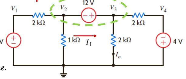
Since this surface is a collection of two nodes with different voltages at both the ends, we refer to this as Super-node.
