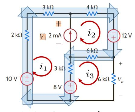
Since this loop is a collection of two loops with different loop currents in these loops, we refer to this as Super-loop. The use of super loop is useful when the current source is shared between two loops.
