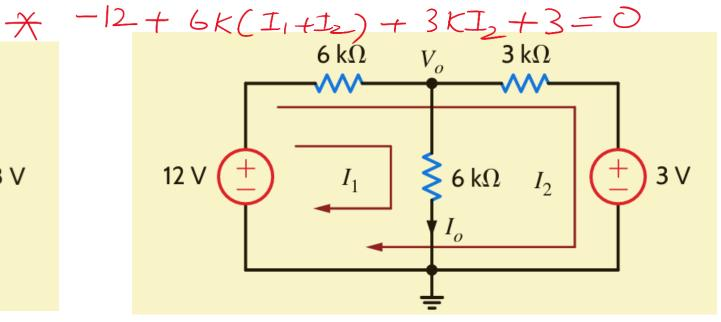
Independent loop: if loop traverses at-least one element that is not part of any other loop
