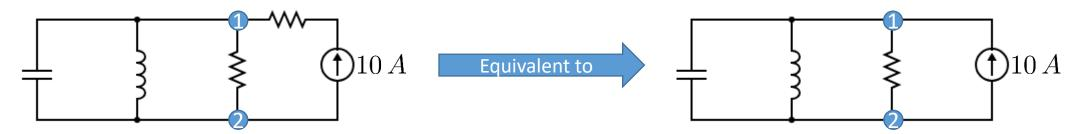
10A is being fed to node 1 and 10A is being drawn from the node 2.
